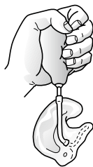
Use air bulb to remove residual water.
